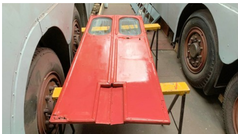
243's folding doors following painting in Hammerite special metals primer.
