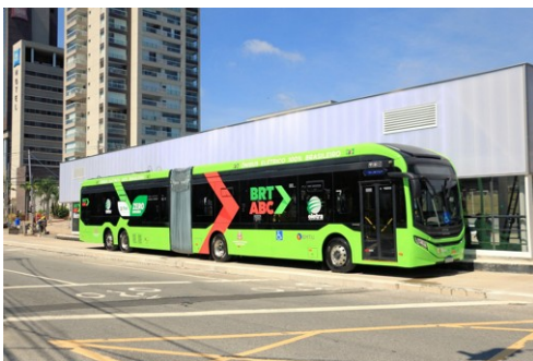
A São Paulo Caio Millennium BRT articulated trolleybus. It is a Mercedes-Benz with Caio Induscar body and Eletra electrical equipment. [BRT ABC]
