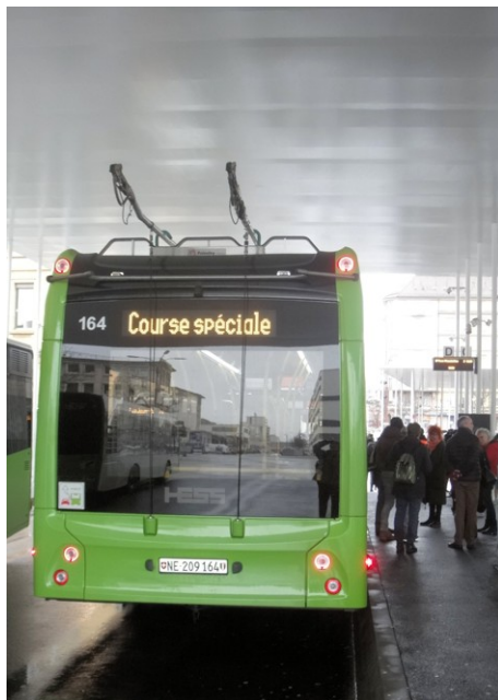
▲ The bus station is unwired, so this section is operated in battery mode. 164 before the start. [David Bowler]
