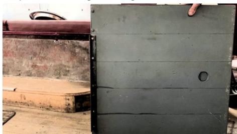
The strengthened hatch board above 243's motor. [Keith Walker]
