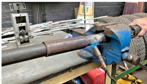
Cardiff 243's nearside boom having heat applied to successfully straighten it. [Keith Walker]
