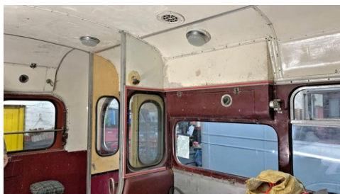
The new Herzim plastic in its aluminium trim around 243's door partition and side destination box. [Keith Walker]
