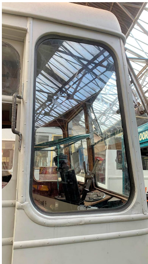
Cardiff 243's driver's cab offside window with its new window rubber. [Keith Walker]
