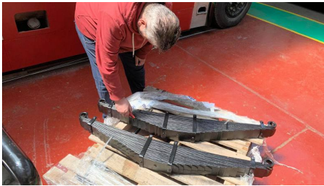
The front springs for 243 have been returned following refurbishment. [Keith Walker]
