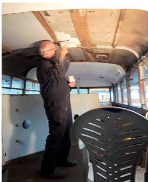
Jeff White applies primer to the inner face of 262's roof panels. [Keith Walker]
